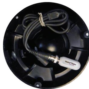
Install a Balun within the base of the camera.
