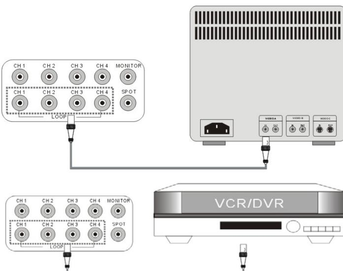
To monitor a single channel, connect the “loop out” of the corresponding channel to a monitor.
