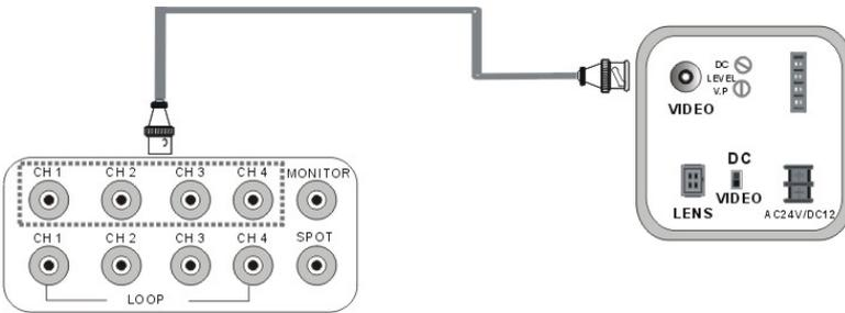
Connect camera to DVR camera in CH1~CH16
