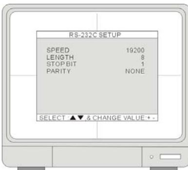
Through the RS232 port, users can connect the DVR to a PC or other control devices to control the DVR. Users cannot change value in this setting.
