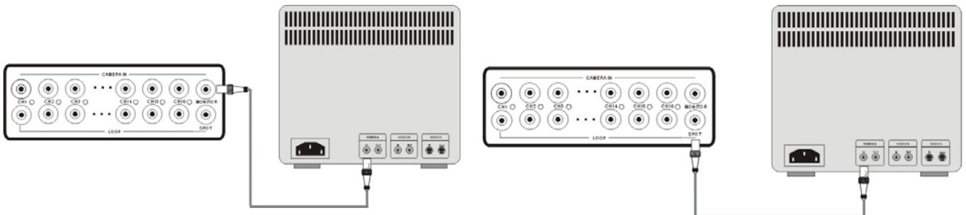
Monitor: Connect the MONTIOR port on the DVR back panel to the “video in” port on the monitor.
