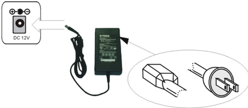
Insert the adapter to the rear power socket of DVR. Insert the power cable to the other side of adapter.
