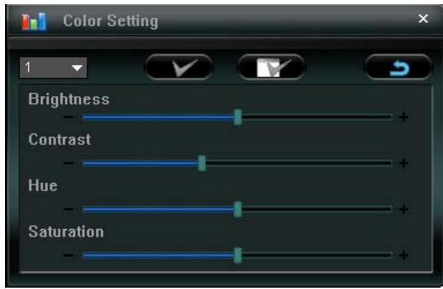
Choose the desired channel from the drop-down list, and click and drag the slider to make adjustment. Click “” to apply the change to the selected channel, or “” to apply to all channels.
