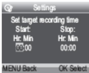
Press the up/down buttons to set the hour for the start of the active phase. Then switch to the next field using the right button to set others.
