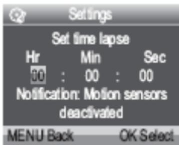
Press the up/ down buttons to set the hour of the desired time interval. Then switch to the next field, “Min”, using the right button. Press the up/down buttons to set the minutes of the desired time interval. Then switch to the next field, “Sec”, using the right button. Press the up/down buttons to set the seconds of the desired time interval.
