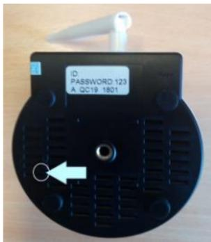
**If after 30 seconds the camera does not start to beep:** Reset the camera by inserting a pin into the RESET hole on the underside of the camera for 5 seconds until the unit makes a noise. Then leave for 30 seconds until the camera beeps.
