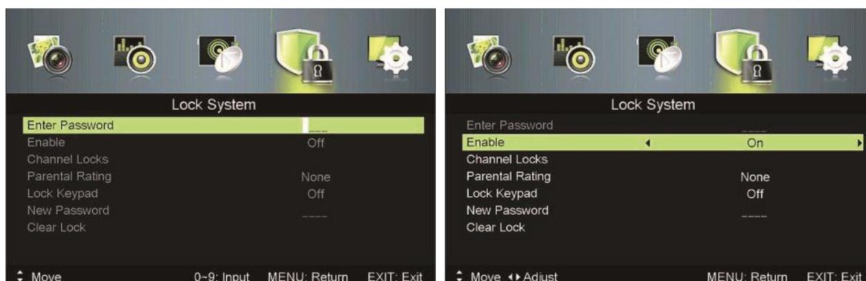
The lock system enables you to put a password on the TV set. The default password is **0000**. To make changes, enter the password and use the ▲ / ▼ to navigate to the required setting. Press the ◀ / ▶ to make the required changes then press the MENU button to return or EXIT to exit.
