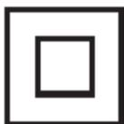
This equipment is a Class II or double insulated electrical appliance. It does not require a grounded connection.
