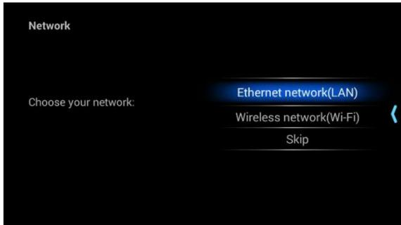
Select Ethernet (LAN) or WIFI as internet connection method. If WIFI signal is weak or you have a router within your reach please use wired connection via RJ45 connector and cat5e or better cable into your router. For connectivity over WIFI please an access point and input the WIFI key via remote or keyboard.
