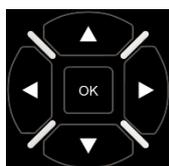
Use arrows to navigate the smart TV menu and **OK** key to select. Basic navigation and text input can be done via those keys. Certain functions will required virtual remote or the optional all-in-one advanced remote. While mouse emulation is off the arrow keys deliver basic scrolling.
