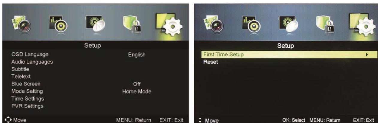
To make changes use the ▲ / ▼ to navigate to the required setting. Press the ◀ / ▶ to make the required changes then press the MENU button to return or EXIT to exit.
