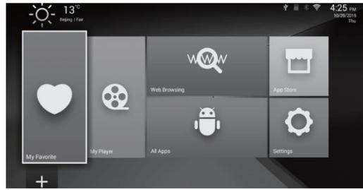
Launcher tab contains: Weather information, Time, Wifi / Wired network, USB connection status (white for connected, gray for standby)
