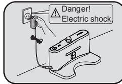
2. Insert the adaptor into the power socket side and another side in the charging station.
