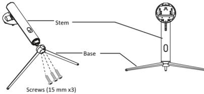
3. Align the stand stem's bracket with the opening on the back of the monitor and carefully insert bracket. The pieces should click into place.
