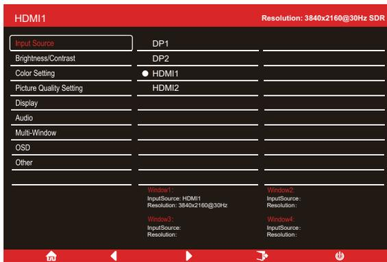
Signal | Switch the signal input or select the source. DP 1, DP2, HDMI1, HDMI2
