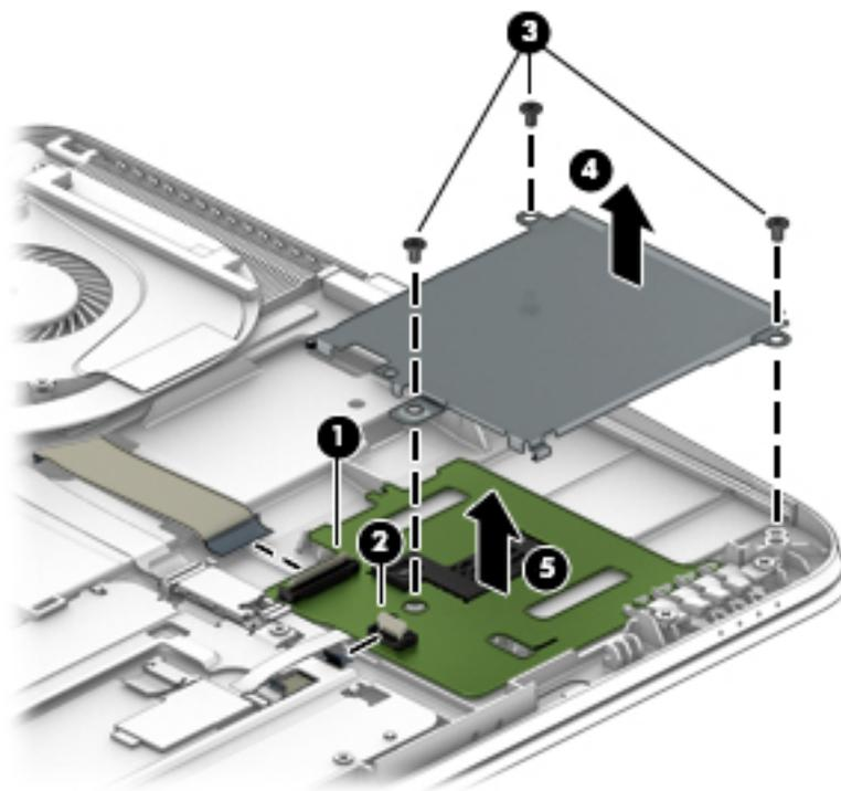
Reverse this procedure to install the smart card reader board.
