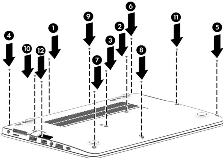
There are four different sizes of rubber screw covers. Be sure that you reinstall them over the correct screws. The rubber-screw cover sizes are as shown in the following image:
