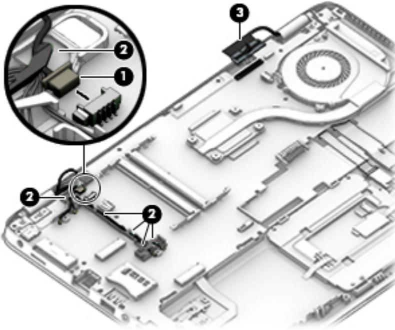
5. Remove the 4 Phillips M2.5×5.0 screws (1) that secure the system board to the computer.
