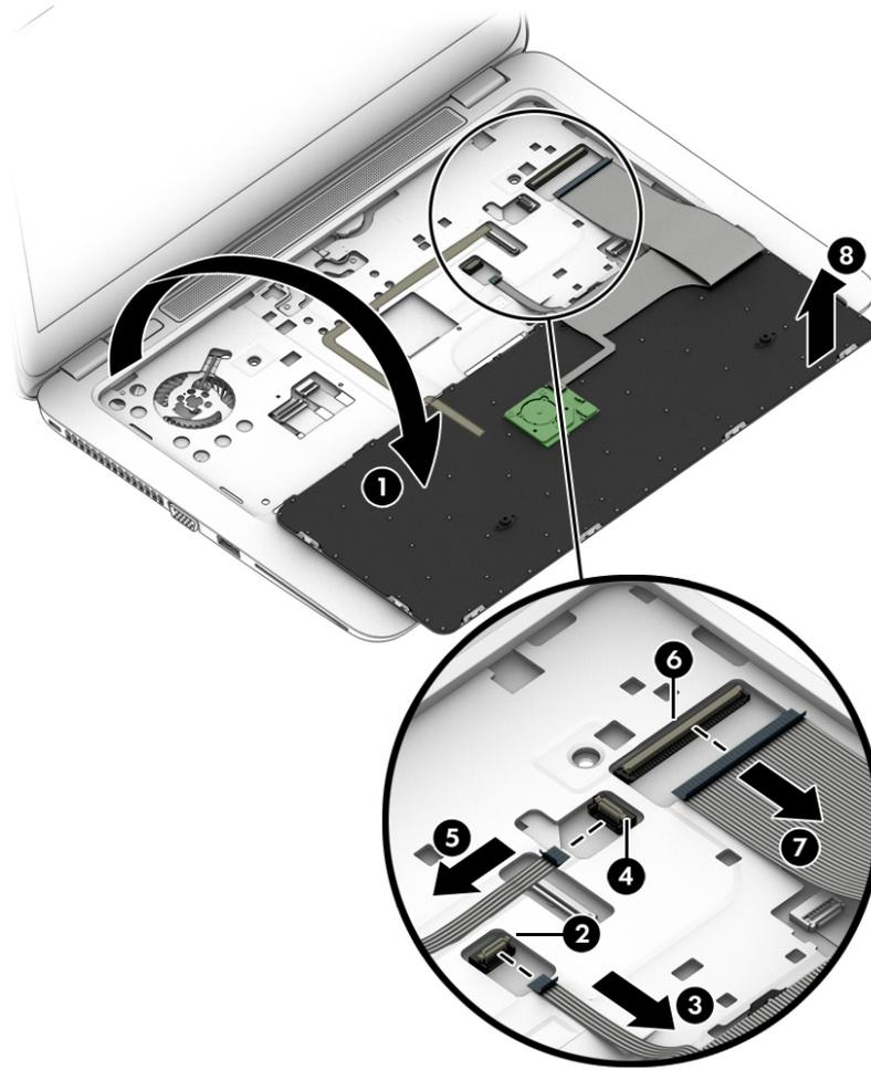
Reverse this procedure to install the keyboard.
