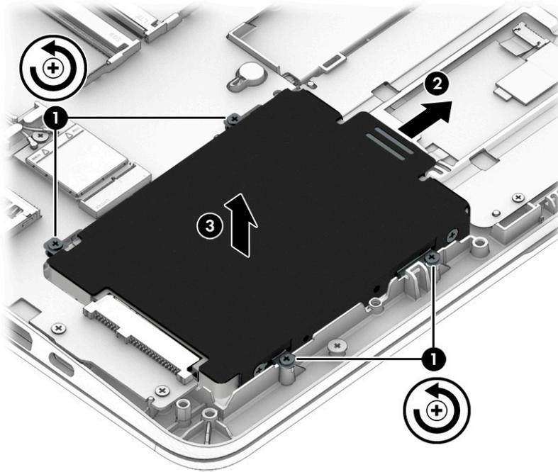
4. To remove the hard drive cover from the hard drive, remove the 4 Phillips M3.0×3.0 screws (1) that secure the bracket to the drive, and then lift the bracket up and off the hard drive (2).
