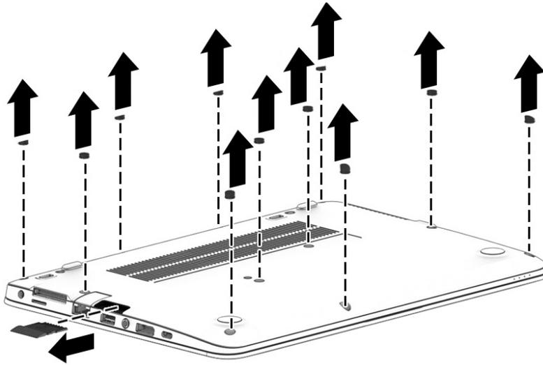
4. In the order indicated in the following image, remove the 12 Phillips M2.5x5.0 screws from the bottom cover.
