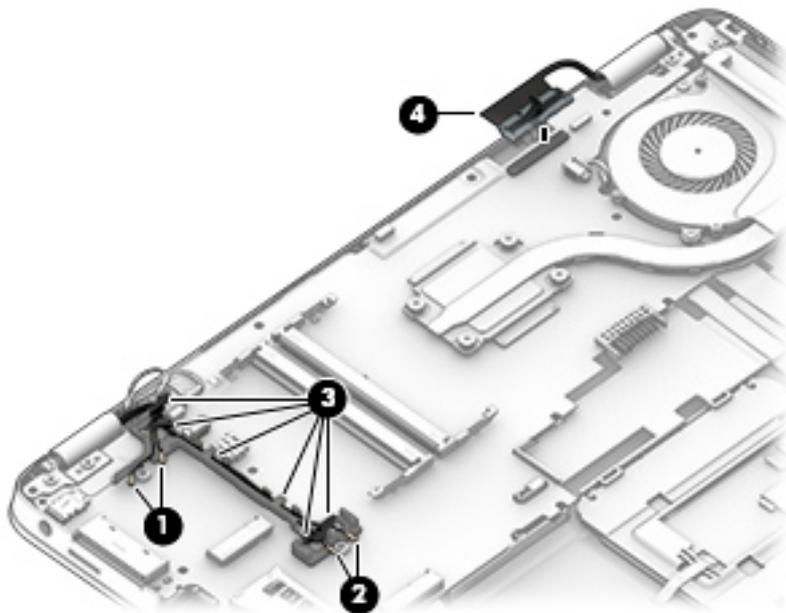
6. Remove the 4 Phillips M2.5×5.0 screws **(1)** from the display hinges.
