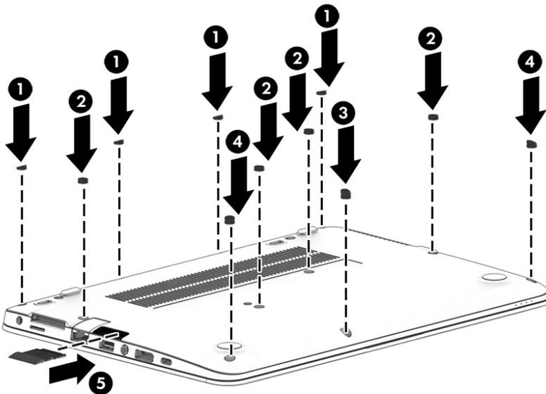
**NOTE:** If installing new rubber screw covers, carefully inspect for adhesive tape liner inside the cap and remove if present.
