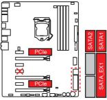
1xM.2 SATA SSD + 1xM.2 PCle SSD + 2xSATA HDDs + 1xSATAe HDD
