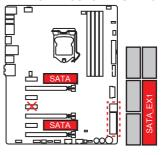
2xM.2 PCIe SSDs + 2xSATA HDDs + 1xSATAe HDD
