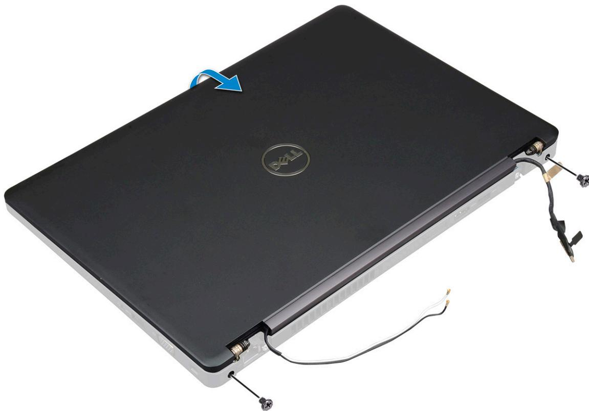
c Lift the display assembly from the computer.
