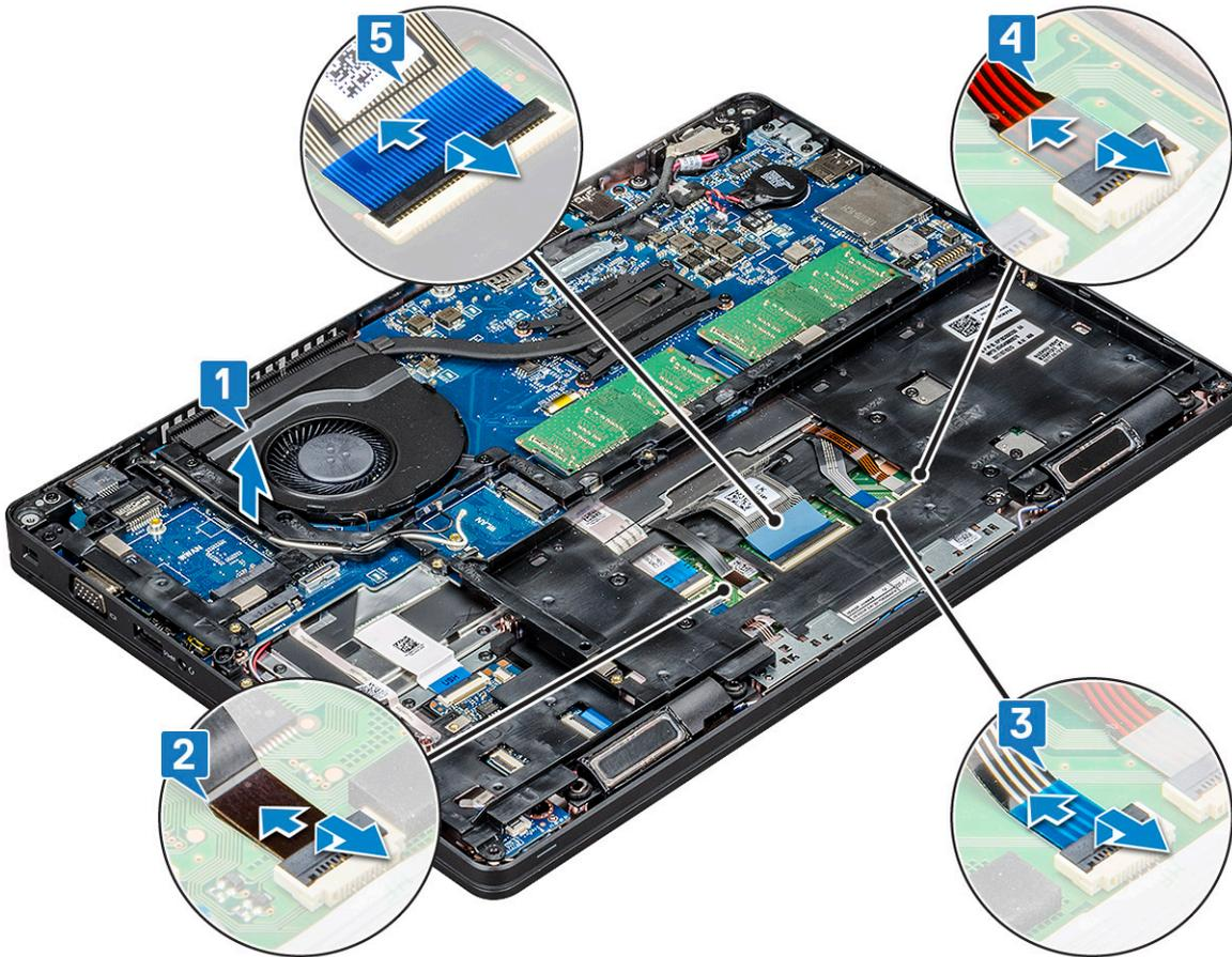
4 To remove the chassis frame:
