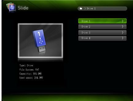
When this happens, use the cursor keys to move the highlighting to the drive you want to use and then press the [ENTER] key. This will display a menu of files for the mode you are entering.
