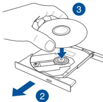
4. Push down the disc's plastic hub until it snaps onto the optical drive hub.
