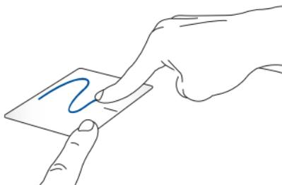
Select an item then press and hold the left button. Using your other finger, slide on the touchpad to drag the item, lift your finger off the button to drop the item.
