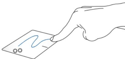
Double-tap an item, then slide the same finger without lifting it off the touchpad. To drop the item to its new location, lift your finger from the touchpad.
