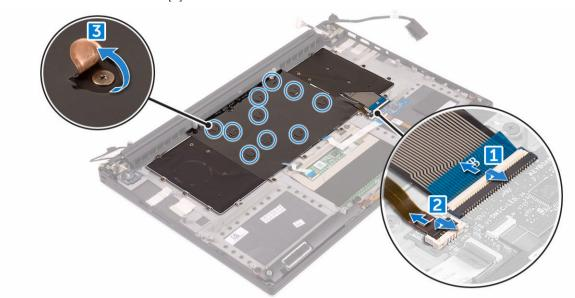
4 Un-route the LVDS cable [1] and then remove the 31 M1.6 x 1.5 screws that secure the keyboard to the computer [2].
