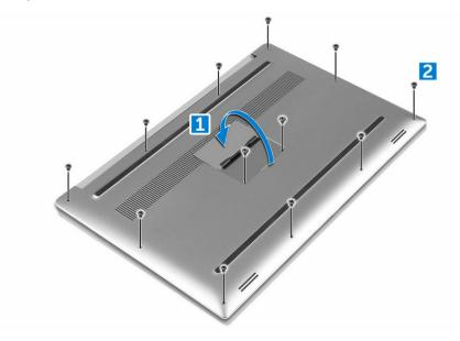
4 Pry the edges of the base cover and lift it to remove it from the computer.
