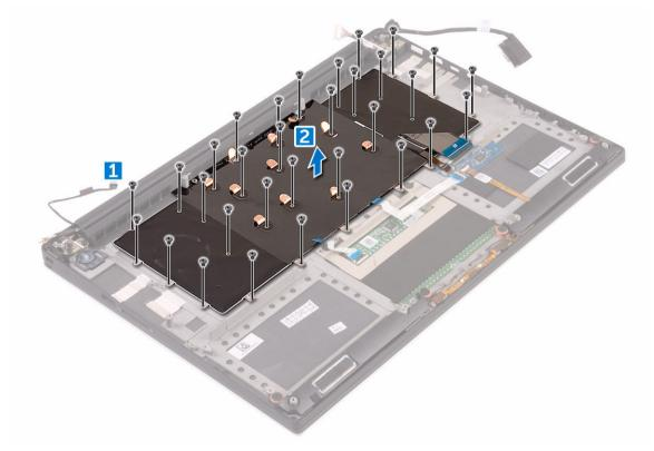
5 Lift and remove the keyboard from the computer.
