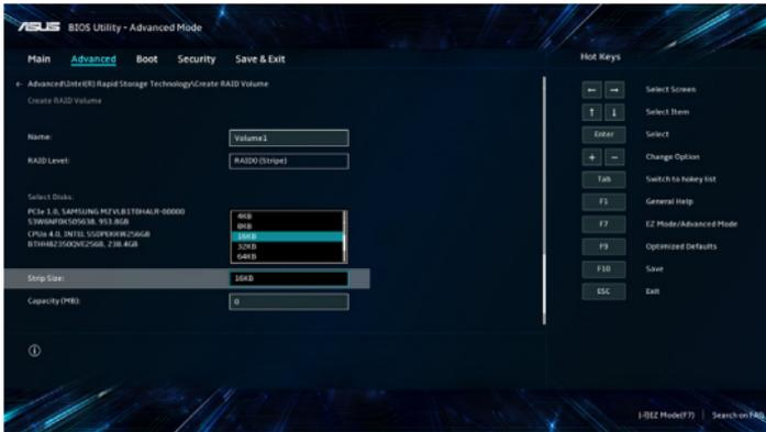
9. When the **Capacity (MB)** item is selected, enter the RAID volume capacity that you want and press <Enter>. The default value indicates the maximum allowed capacity.
