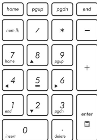
A numeric keypad is available on selected Notebook PC models. You can use this keypad for numeric input or as pointer direction keys.
