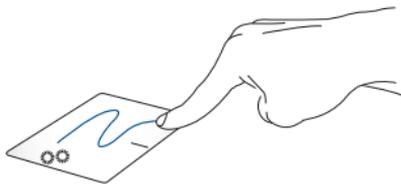
Double-tap an item, then slide the same finger without lifting it off the touchpad. To drop the item to its new location, lift your finger from the touchpad.
