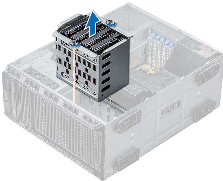
**Figure 37. Removing the internal hard drive bay**
