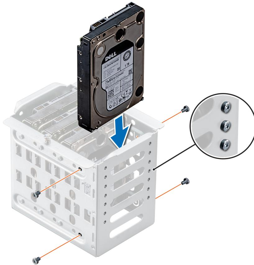
Figure 40. Installing a cabled drive
