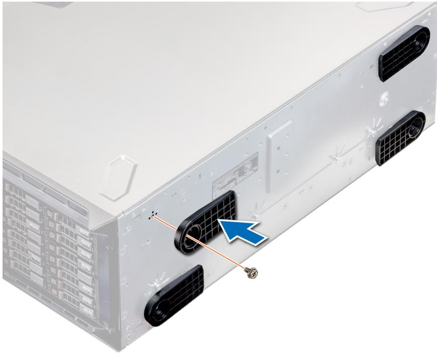
**Figure 16. Installing the system feet**
