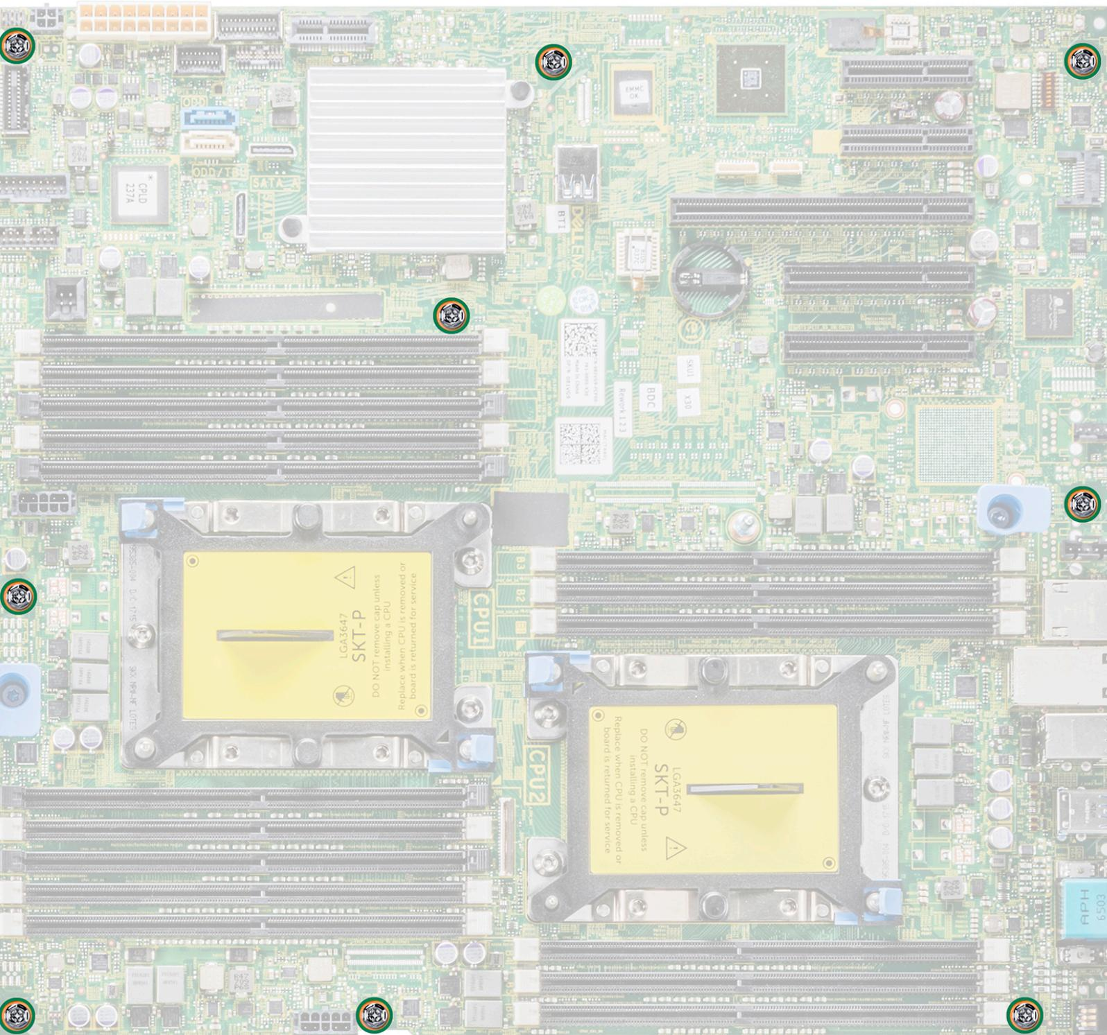
Figure 84. System board screws
