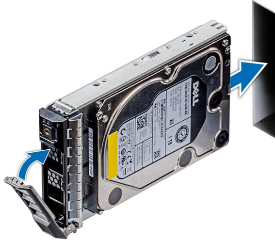
Figure 26. Installing a drive carrier
