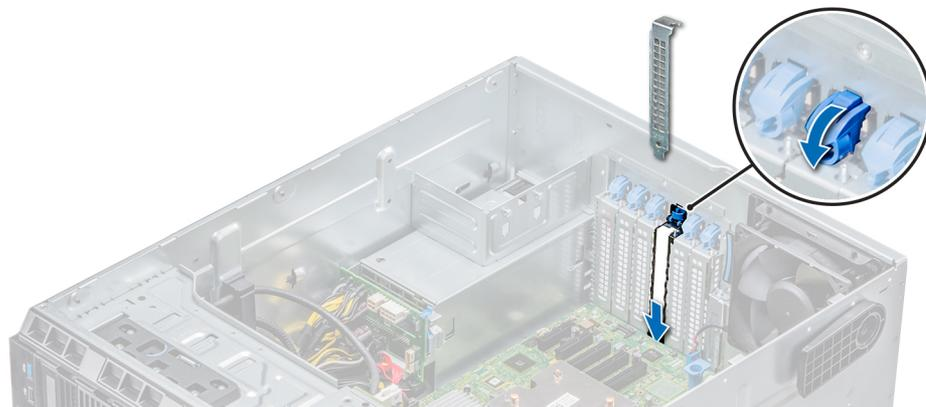
**Figure 59. Installing the filler bracket**
