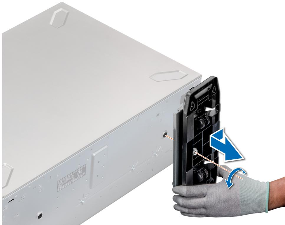
**Figure 17. Removing caster wheels**
