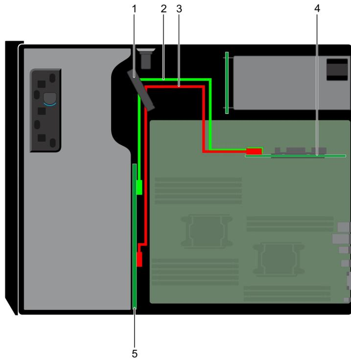
**Figure 46. Cable routing - 8 x 3.5 inch drive backplane with internal PERC**
