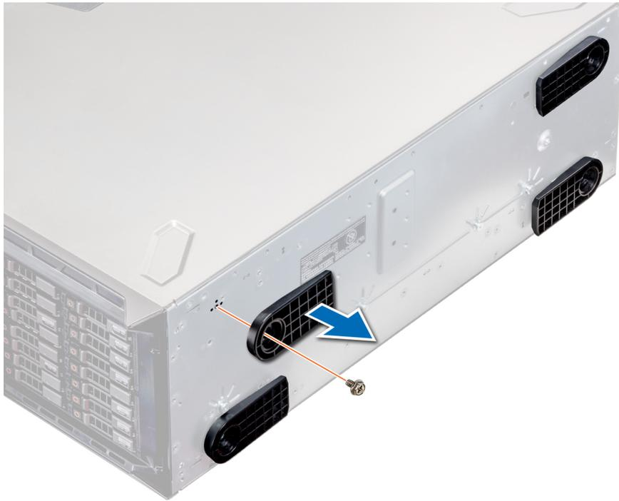
**Figure 15. Removing the system feet**
