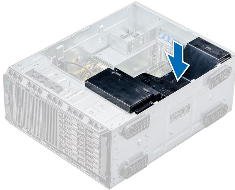
**Figure 22. Installing the air shroud**
