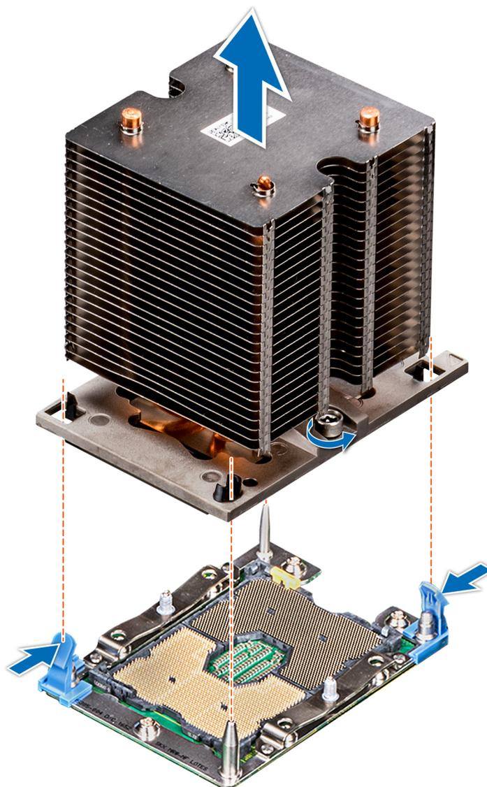
Figure 64. Removing the processor and heat sink module
