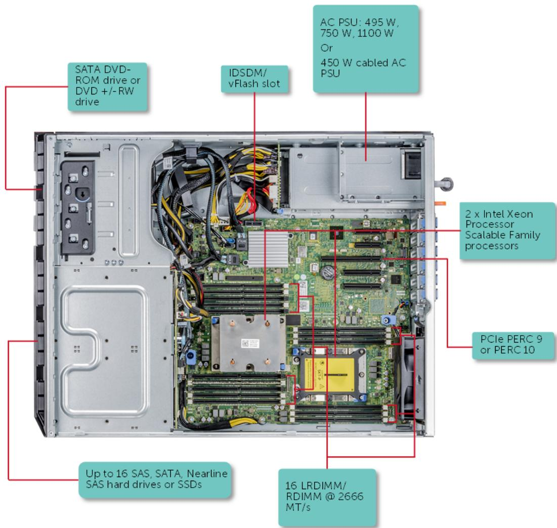
Figure 1. Supported configurations for a PowerEdge T440 system
