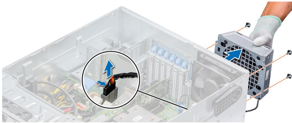
**Figure 54. Removing the external cooling fan**
