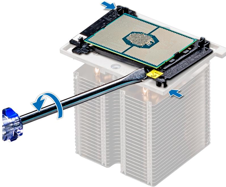
**Figure 65. Loosening the processor bracket**
