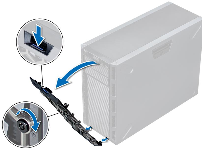
Figure 13. Removing the front bezel
