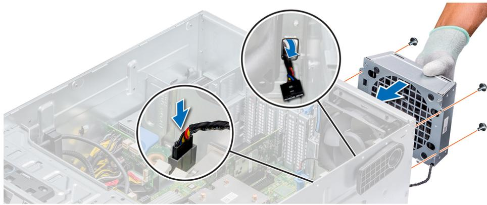
**Figure 55. Installing the external cooling fan**
