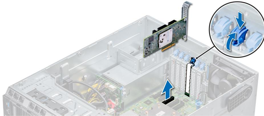
**Figure 58. Removing an expansion card**
