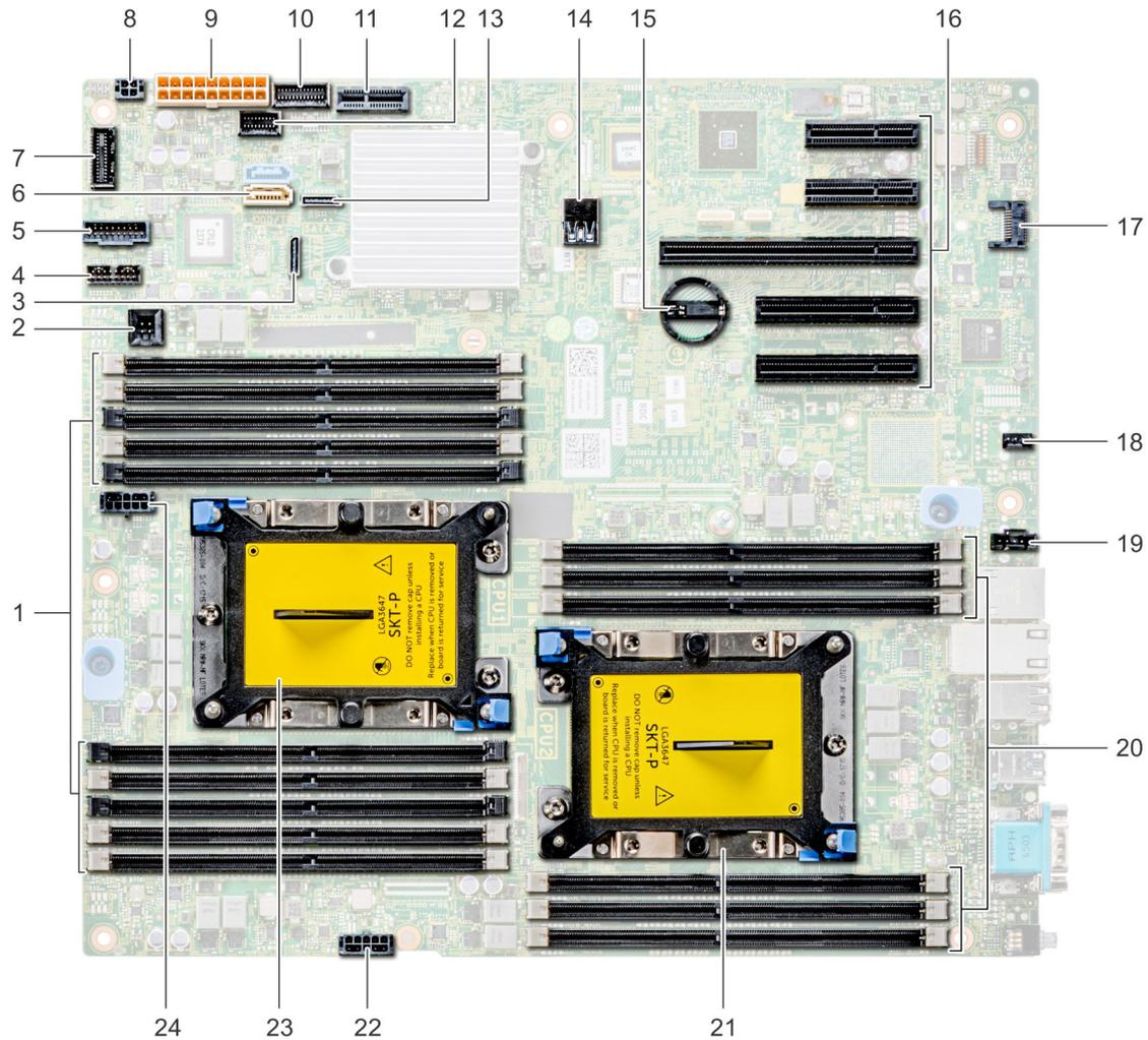
Figure 89. T440 System board jumpers and connectors
