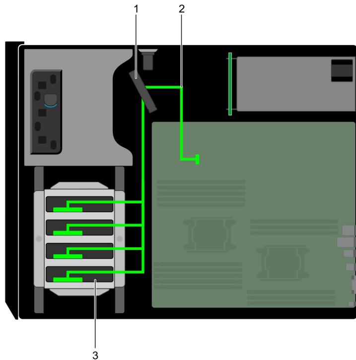
**Figure 48. Cable routing - 4 x 3.5 inch cabled HDD**
