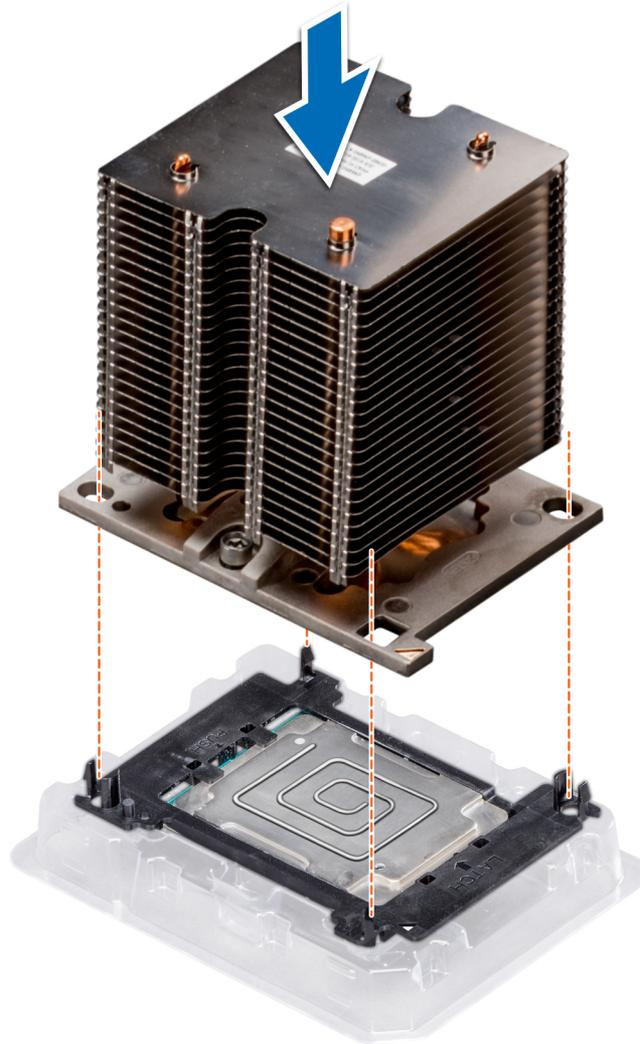
**Figure 69. Installing the heat sink onto the processor**
