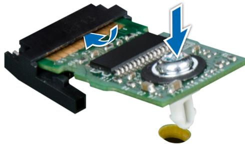
Figure 87. Installing the TPM
