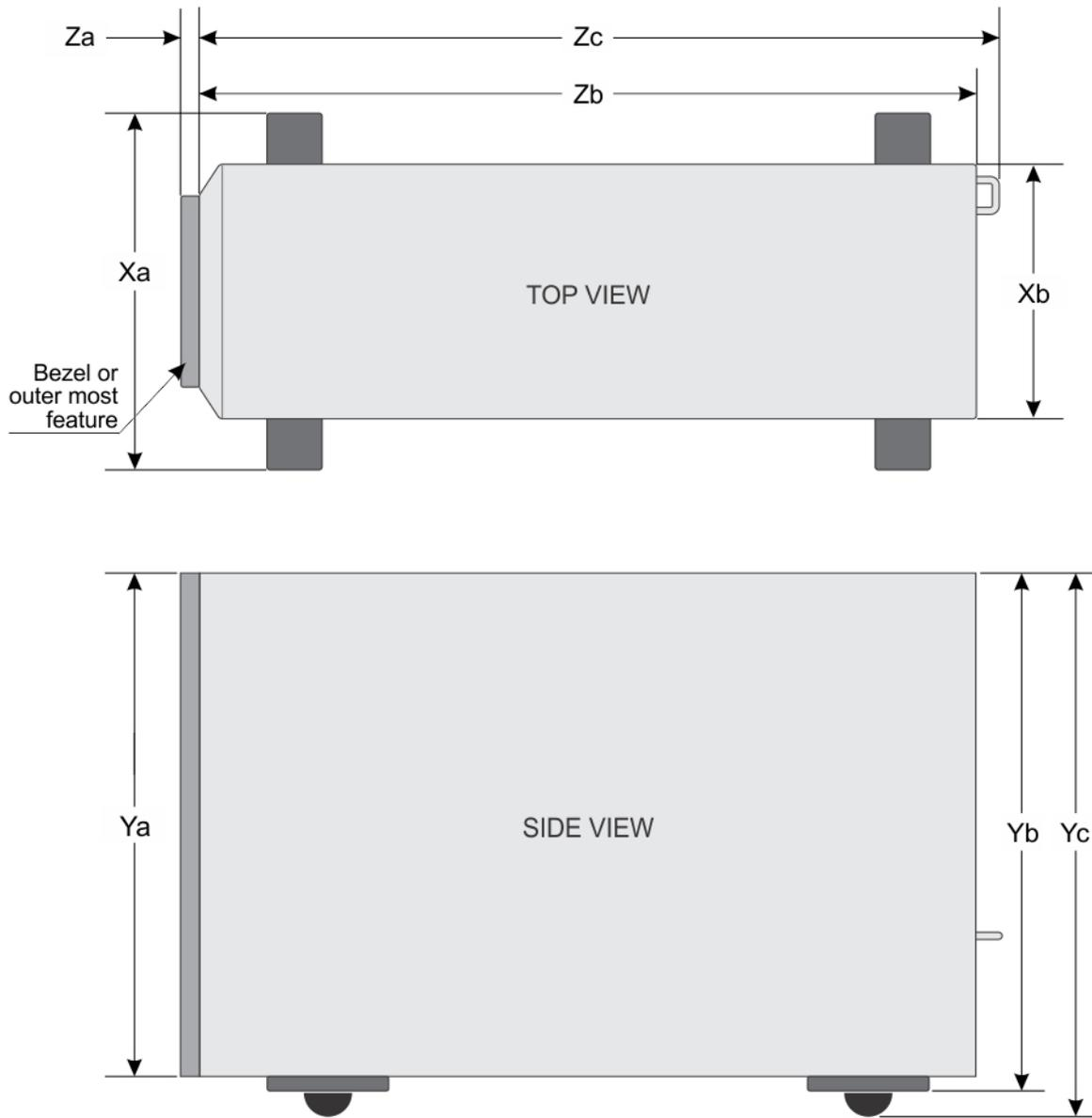
Figure 12. Details the dimensions of the PowerEdge T440 system
