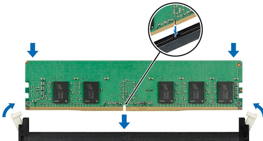
Figure 51. Installing a memory module
