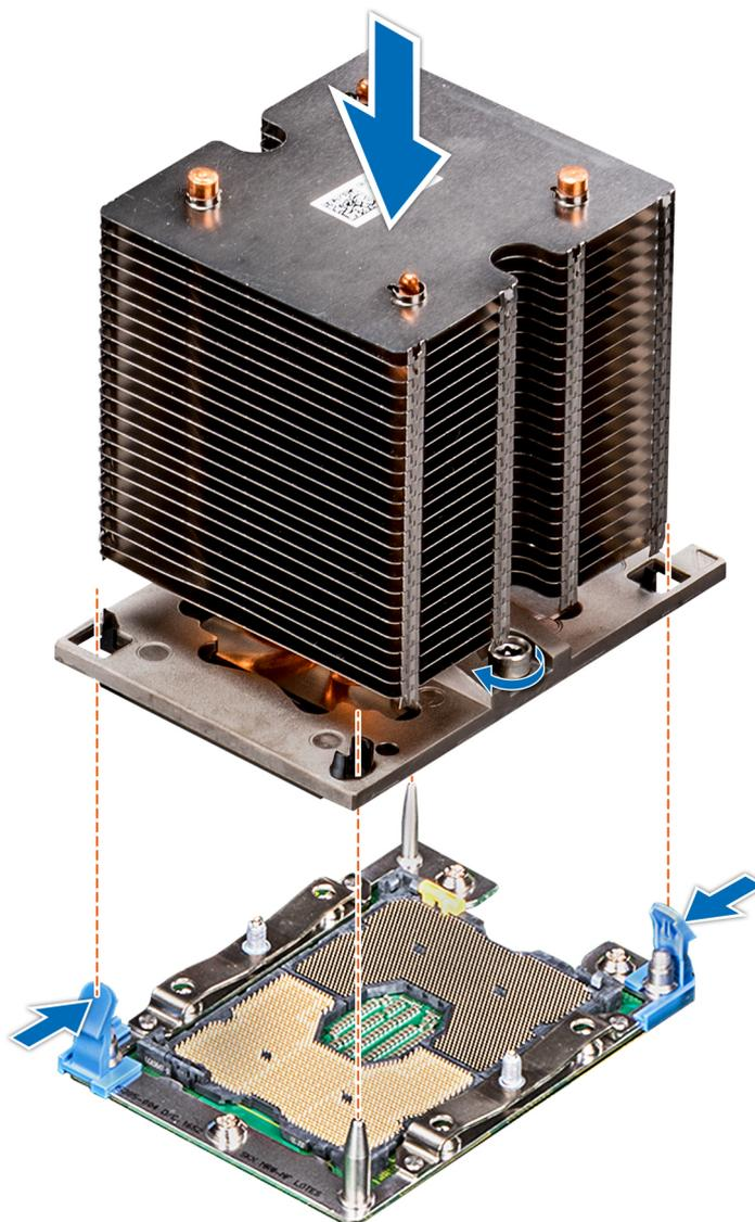
Figure 70. Installing a processor and heat sink module
