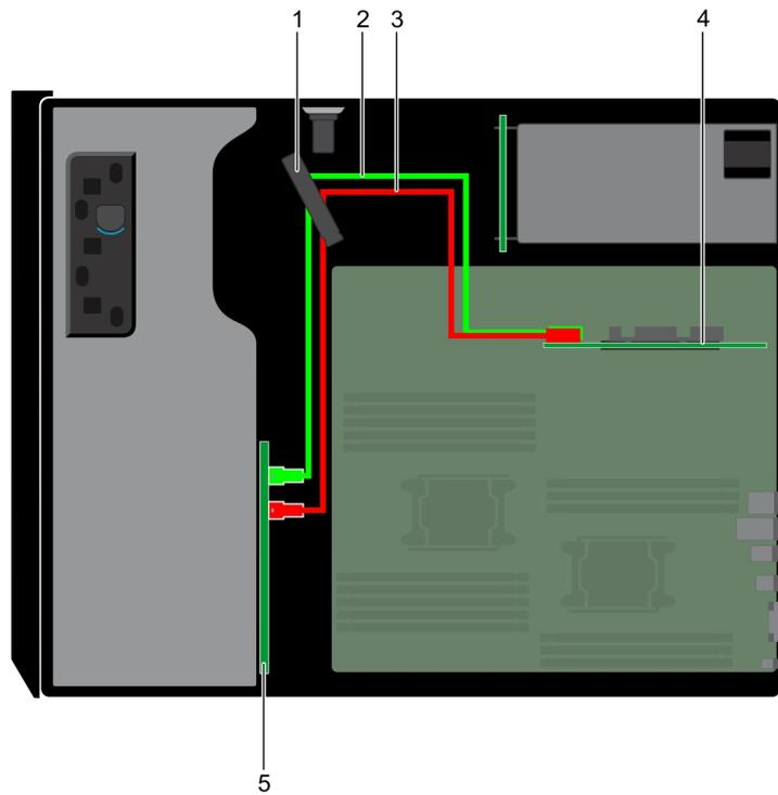
**Figure 47. Cable routing -16 x 2.5 inch drive backplane with internal PERC**
