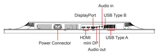
3.A. Please do not connect the DisplayPort out on the monitor to the DisplayPort or mini DP connector on the computer. DisplayPort out is used for daisy chain connection (Explained in section D)
