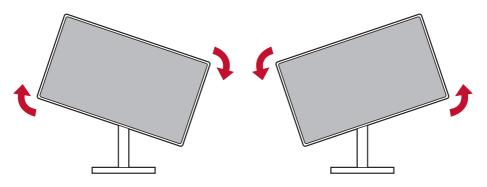
4. Finish the monitor installation by fully rotating the monitor 90°(see the below picture for reference).
