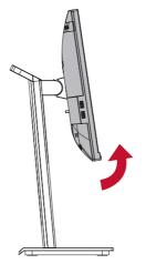
3. Rotate the monitor clockwise and counterclockwise, (see the below picture for reference).
