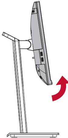
3. Rotate the monitor clockwise and counterclockwise, (see the below picture for reference).
