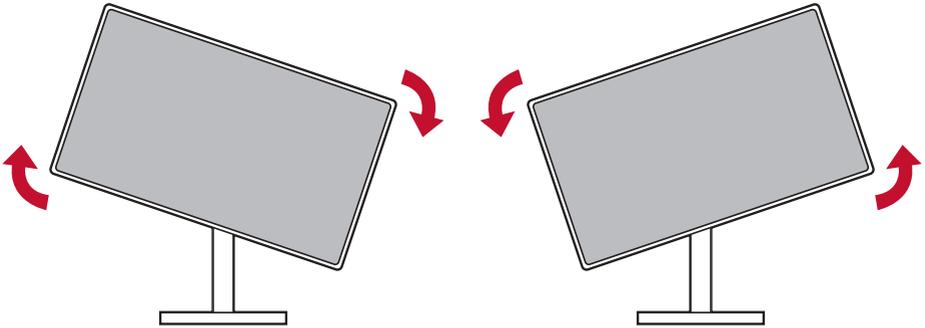
4. Finish the monitor installation by fully rotating the monitor 90°(see the below picture for reference).
