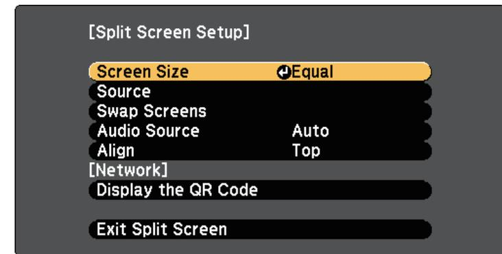
**3** To select an input source for the other image, select the **Source** setting, press [Enter], select the input source, select **Execute**, and press [Enter].
