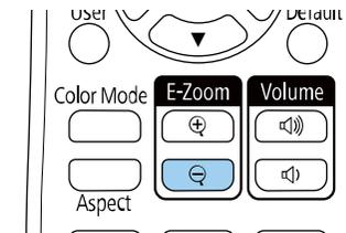
The projected image is reduced. You can reduce the image between 100% to 50% in incremental steps.
