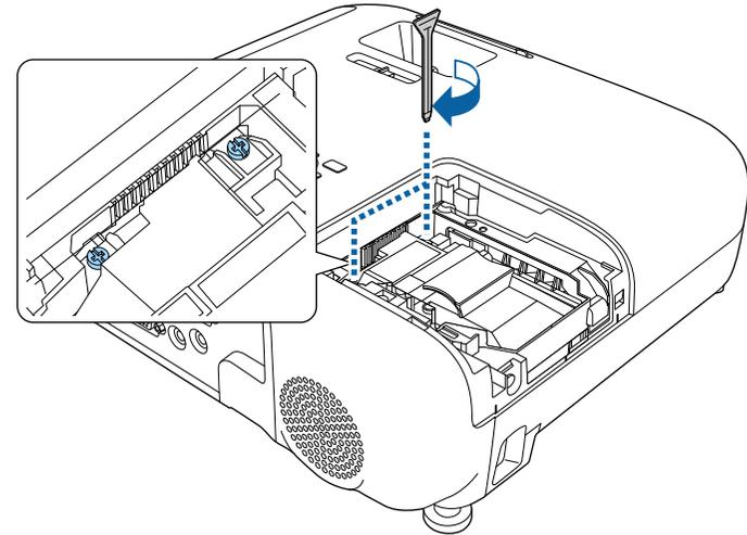
**9** Replace the lamp cover and tighten the screw to secure it.
