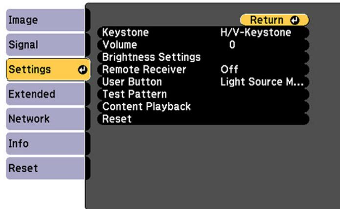
**Note:** You can also press the **Keystone** button on the remote control to display the Keystone adjustment screen.
