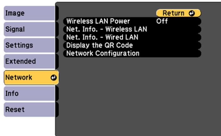
4. Select **On** as the **Wireless LAN Power** setting and press **Esc**.
