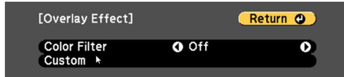
4. Select **Color Filter**, press **Enter** (↵), and use the left and right arrow buttons to select a color for the overlay effect. Press **Menu** to exit.
