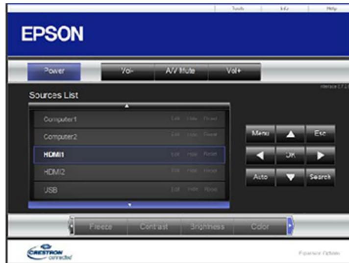
4. Select the input source that you want to control in the Sources List box. You can scroll through available sources using the up and down arrows in the box.
