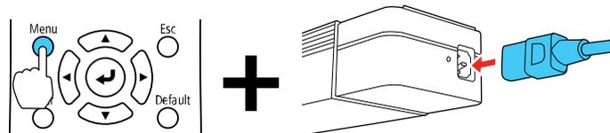
4. When the On/Standby and Status lights are blue, and the Laser and Temp lights are orange, release the **Menu** button.
