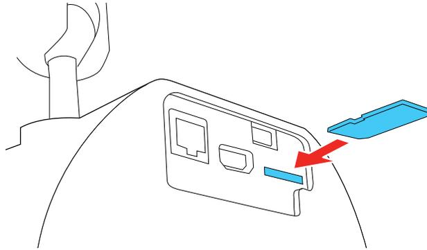
**Note:** Insert the SD card directly into the projector. Do not use a hub or your settings may not transfer correctly.
