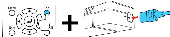
4. When the On/Standby and Status lights are blue, and the Laser and Temp lights are orange, release the **Esc** button.
