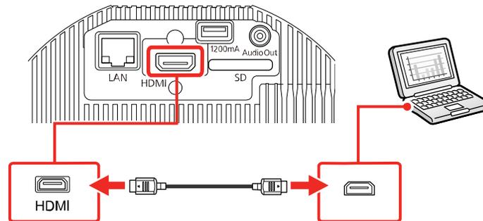
**Note:** The projector converts the digital audio signal sent from your computer into a stereo analog signal if you are connecting to external speakers. (Make sure the HDMI audio playback device on your computer's audio settings is set to **EPSON PJ.**)
