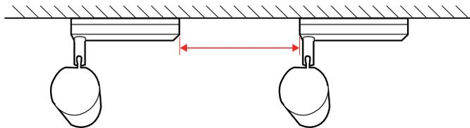
You can rotate the projection unit 360 degrees horizontally and 90 degrees vertically. You can also tilt the image 90 degrees in either direction.
