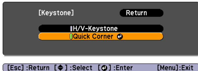
**4** Using the [⏪], [⏩], [⏴], and [⏵] buttons on the remote control, or the [△], [▽], [←], and [→] buttons on the control panel, select the corner to correct, and then press the [↵] button.
