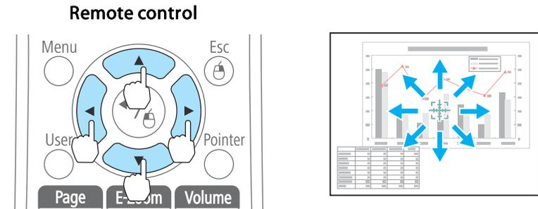
When any pair of adjacent [◀], [▶], [⏪], or [⏩] buttons are pressed at the same time, the pointer can be moved diagonally.
