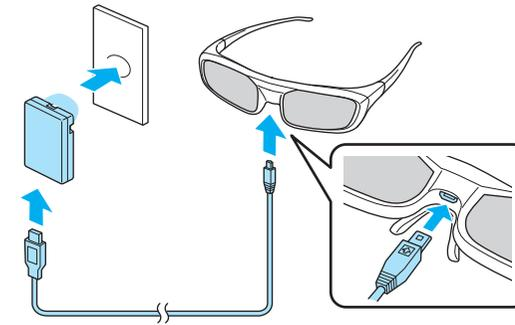
You can also charge the 3D Glasses by connecting the charging cable supplied with the glasses to the USB(TypeA) port on the rear of the projector. (Charging only works when the projector is on.)
