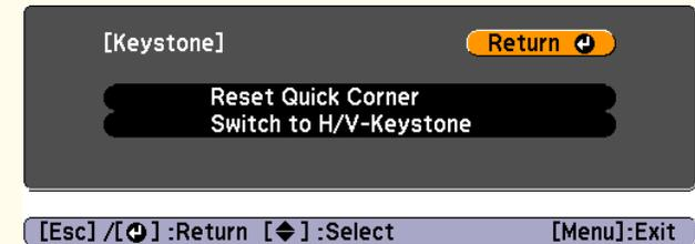
**Reset Quick Corner:** Resets the result of Quick Corner corrections.
