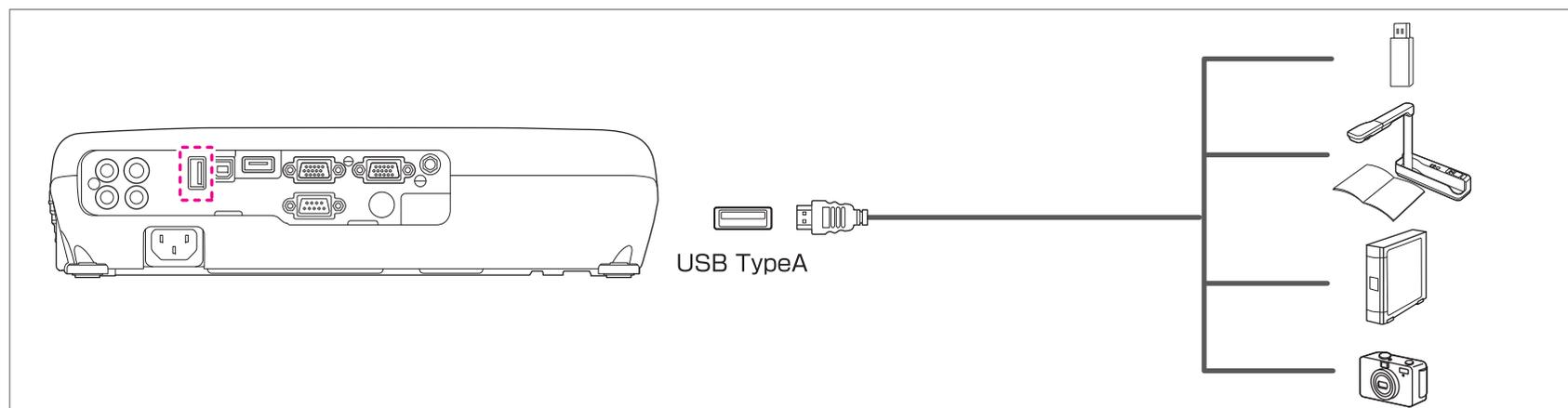
When the USB device is connected, you can project files on the USB memory or digital camera using PC Free.
