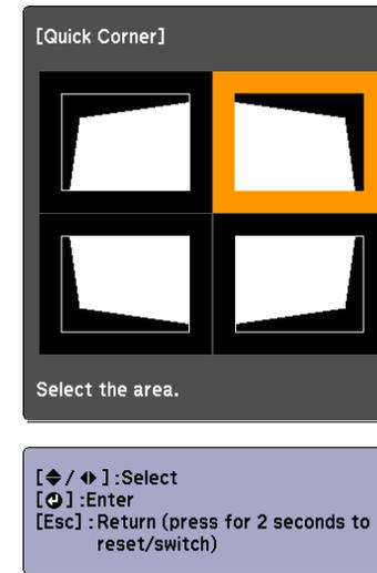
**5** Using the [⏪], [⏩], [⏴], and [⏵] buttons on the remote control, or the [△], [▽], [←], and [→] buttons on the control panel, correct the position of the corner.
