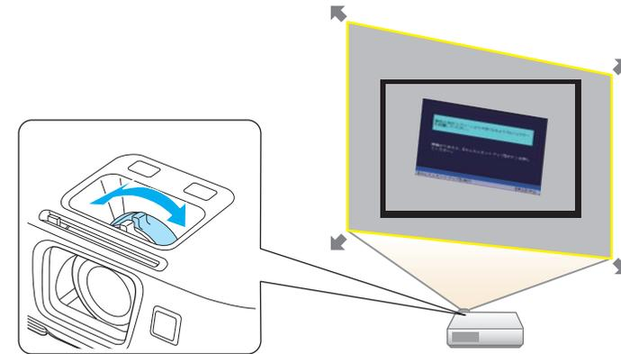
If the yellow frame is still within the screen frame even after adjusting the zoom ring to its maximum size, try moving the projector further away from the screen.
