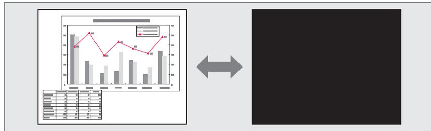
Each time you press the [A/V Mute] button or open/close the lens cover, A/V Mute turns on or off.
