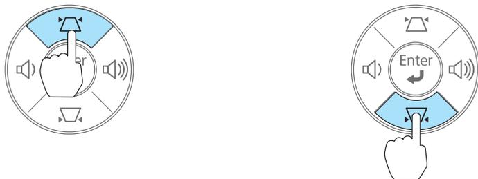
Press the [↔] or [↔] button to correct horizontal distortion.
