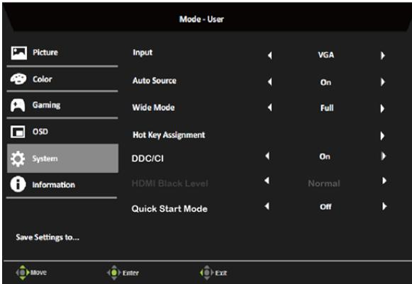
1. The System menu can be used to select settings such as Input, Wide Mode, and Power LED.
