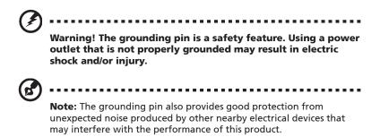
Use the product only with the supplied power supply cord set. If you need to replace the power cord set, make sure that the new power cord meets the following requirements: detachable type, UL listed/CSA certified, type SPT-2, rated 7 A 125 V minimum, VDE approved or its equivalent, 4.6 meters (15 feet) maximum length.
