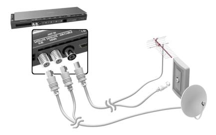
It is best to connect the both connectors using a Multi-Switch or Diseqc. Switch, etc and to set **Aerial Connection Type** to **Dual**.
