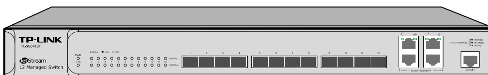
Figure 2-2 Front Panel of TL-SG5412F
