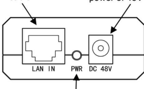
**PWR:** Power LED, a steady green light indicates that the power adapter is working properly.
