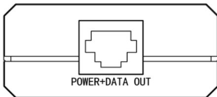
**POWER+DATA OUT:** Connect to the PD or PoE Receiver Adapter with a CAT5 UTP cable.
