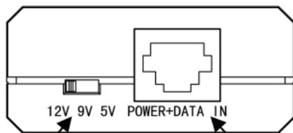
**Power-mode switch:** You can choose the DC output of 12V, 9V or 5V by turning the switch to the left or right.
