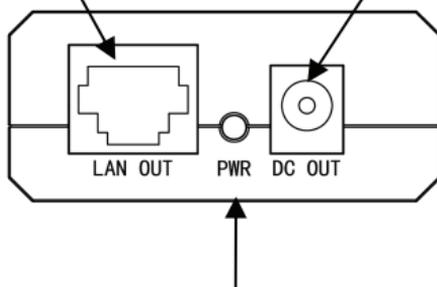
**PWR:** Power LED, a steady green light indicates that the PoE Injector can supply power.
