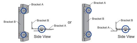
② Depending on the monitor orientation (portrait or landscape) you choose, mount the L-Brackets to the left and right hand sides or the upper and lower sides of the monitor and tighten them with screws supplied (2 pairs of 2 pcs).
