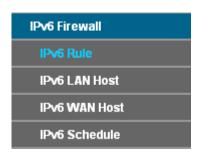
There are four submenus under the IPv6 Firewall menu: IPv6 Rule, IPv6 LAN Host, IPv6 WAN Host and IPv6 Schedule. Click any of them, and you will be able to configure the corresponding function.
