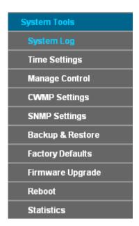
Choose menu "System Tools", and you can see the submenus under the main menu: System Log, Time Settings, Manage Control, CWMP Settings, SNMP Settings, Backup & Restore, Factory Defaults, Firmware Upgrade, Reboot and Statistics. Click any of them, and you will be able to configure the corresponding function. The detailed explanations for each submenu are provided below.
