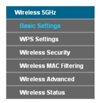
There are five submenus under the Wireless menu (shown in Figure 4-13): **Wireless Settings**, **WPS**, **Wireless Security**, **Wireless MAC Filtering**, **Wireless Advanced** and **Wireless Statistics**. Click any of them, and you will be able to configure the corresponding function.
