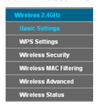
There are six submenus under the Wireless menu: **Basic Settings**, **WPS Settings**, **Wireless Security**, **Wireless MAC Filtering**, **Wireless Advanced** and **Wireless Status**. Click any of them, and you will be able to configure the corresponding function.
