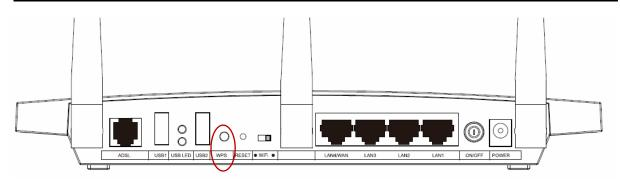
You can also keep the default WPS Status as **Enabled** and click the **Add device** button in Figure 4-41, then Choose "**Press the button of the new device in two minutes**" and click **Connect**. (Shown in the following figure)
