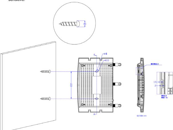
Figure 2-1 Wall-mount install
