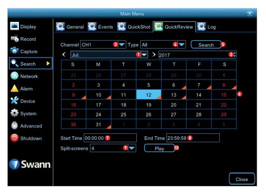
QuickReview allows you to play multiple normal recordings and motion events simultaneously from a single channel. With normal and event recordings, the video is divided evenly depending on the split-screen mode that has been selected. For example, if the video is an hour long and you have selected Split-screens x 4, each split-screen will play for 15 minutes.
