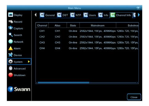
Displays the Mainstream, Substream and Mobilestream settings used for each camera connected.
