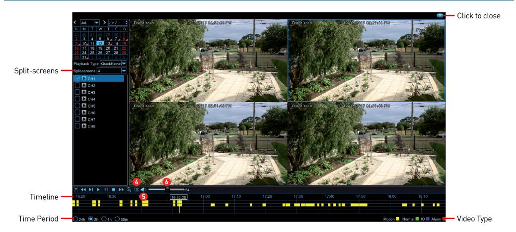
4. This button allows you to edit the video by setting mark in and out points on your video which you can then copy to a USB flash drive. When you have selected a video to play, press this button at the mark in point and press it again at the mark out point. Press the button again to save (a disk icon will be shown). For the backup type, leave the default selection or change to AVI or MP4 for
