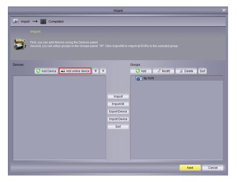
**2.** To display your NVR connected to your router, click the "Add online device" button as shown above (if your NVR does not appear, check that your device is connected to your router using the supplied Ethernet cable).
