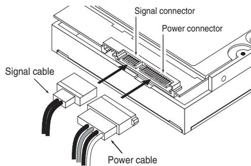
Each cable is keyed to ensure correct orientation. FireCuda drives support latching SATA connectors.
