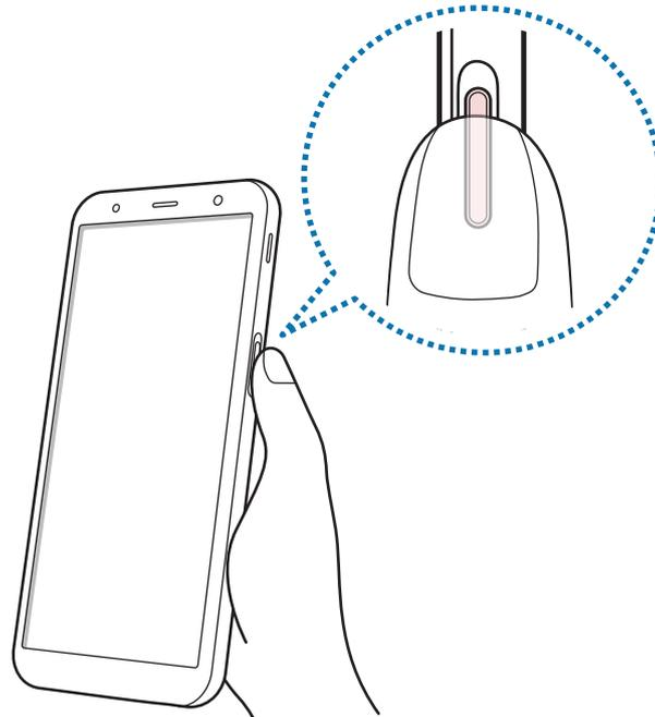
After the device detects your finger, lift it up and place it on the Power key again.
