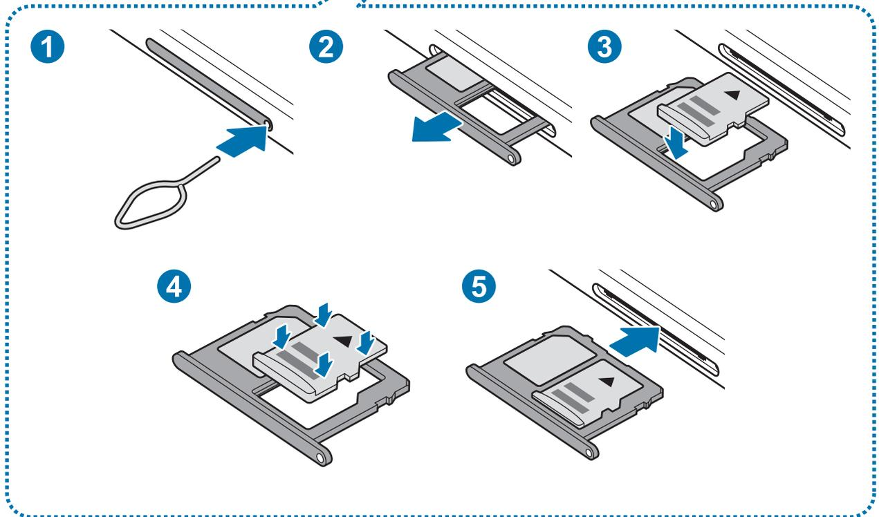
1 Insert the ejection pin into the hole on the tray to loosen the tray.
