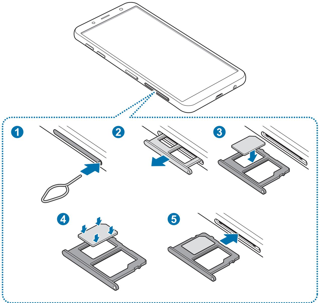
**1** Insert the ejector pin into the hole on the tray to loosen the tray.
