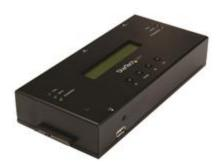
This standalone drive duplicator and eraser supports both SATA and SAS drives, making it a great fit for enterprise storage and data center applications. Compatible with 2.5" and 3.5" drive form factors, it provides a versatile and cost-effective drive management solution.
