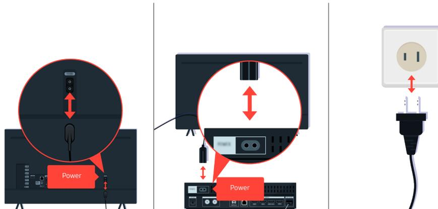
First disconnect and reconnect the power cables and HDMI cables on the back of your TV or the One Connect Box, then unplug the power cable and plug it back into the wall outlet.
