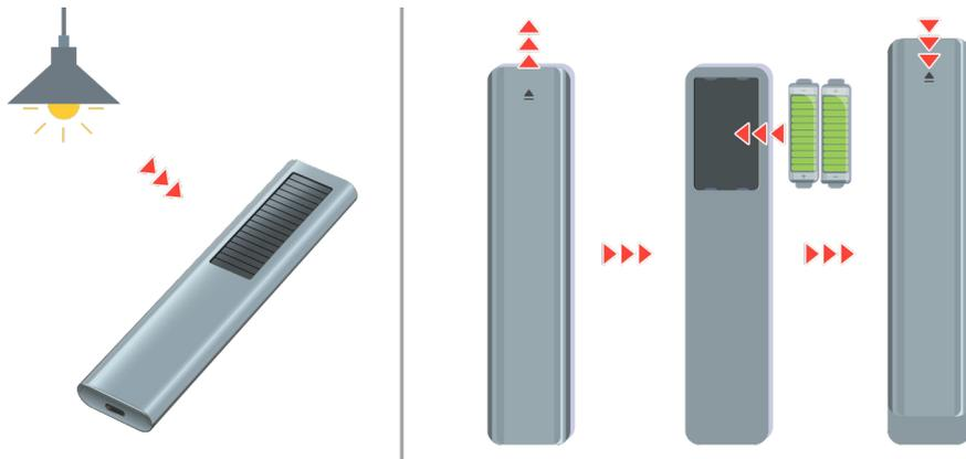
If you cannot see infrared signals, charge the remote control by using the solar cell or the USB port (C-type) on the bottom. If the remote control has batteries, replace them with new ones.
