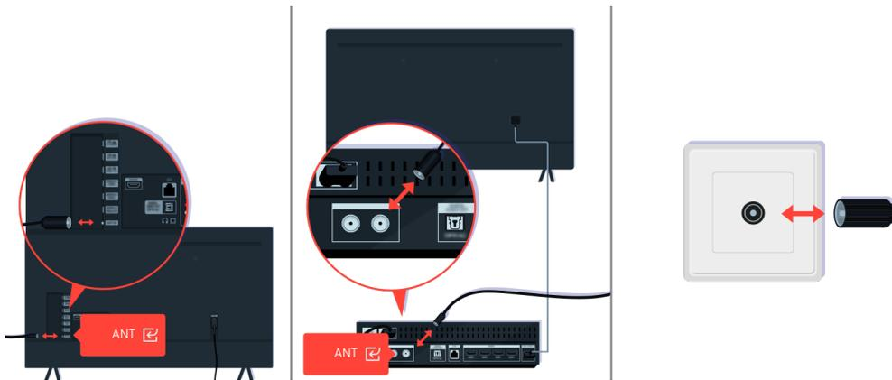
Check the antenna and input cable connections.
