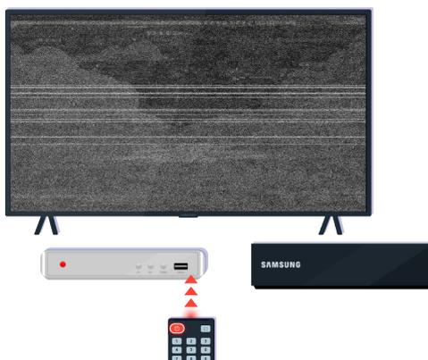
If you use an Multi-Brand Remote (MBR) or universal remote and your remote cannot operate an external device, move the external device closer to the One Connect Box.
