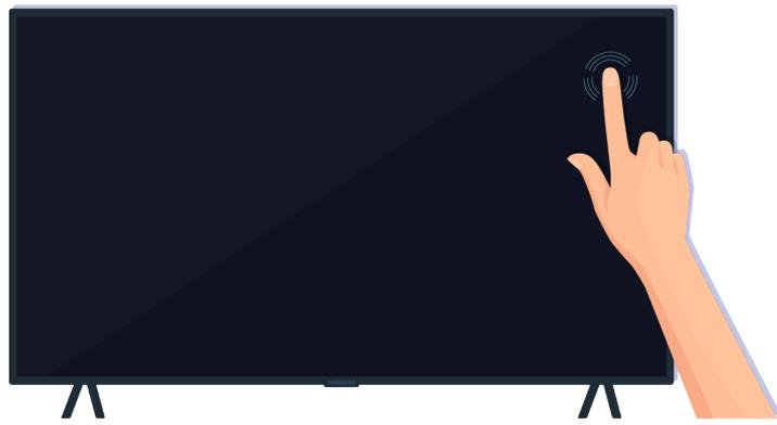
If the TV screen is still blank, softly tap it with your finger. If the part of the screen you tapped on blinks, your TV is correctly connected to the power supply.
