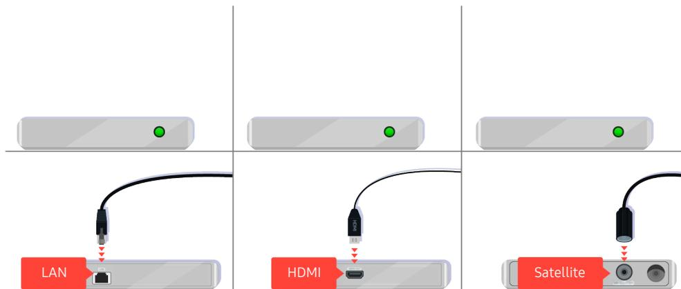
If you are using a set-top box, check the cable connection. The cable you need to check depends on the type of set-top box.
