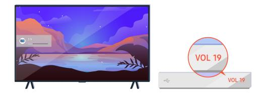
If your TV is connected to an external device, check the volume of the external device.
