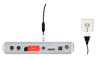
If it does not turn on, make sure the power cable is properly connected to the device and to the wall outlet.
