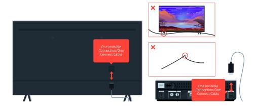
If the problem persists and if your TV uses the One Invisible Connection or One Connect Cable, disconnect and reconnect the One Invisible Connection or One Connect Cable to the TV and the One Connect Box. Ensure that the One Invisible Connection or One Connect Cable is not pinched or bent sharply.
