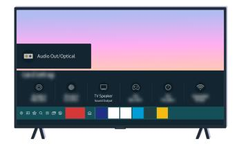
Check the volume on the screen. If a number for the TV volume is not displayed, select > Sound > Sound Output. Then, select TV Speaker.
