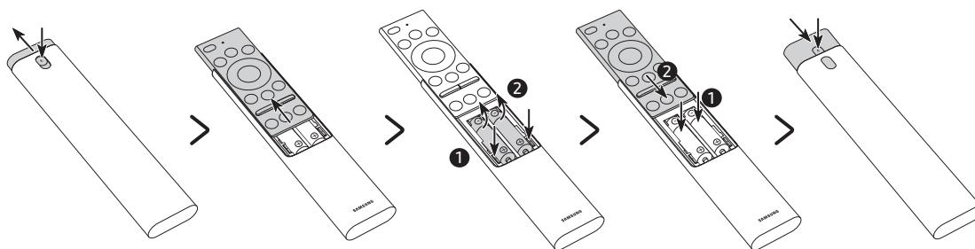
1. Press the ▲ button at the top rear of the Samsung Smart Remote. The body will pop out slightly from the body cover.
