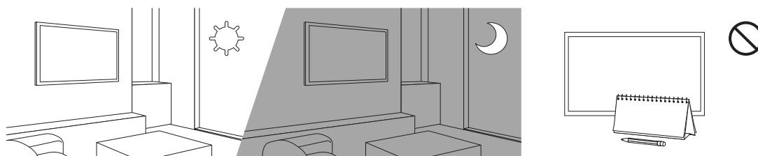
Eco Sensor adjusts the brightness of the TV automatically. This feature measures the light in your room and optimises the brightness of the TV automatically to reduce power consumption.
