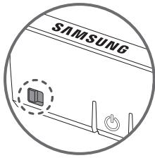
You can turn on or off the sound sensor by using its button at the bottom of the TV. With the TV on, you can push the button to the left to turn on the sound sensor or to the right to turn off it.
