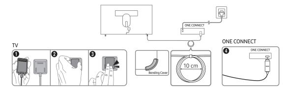
To connect the One Invisible Connection cable to the One Connect and your TV, take the following steps:
