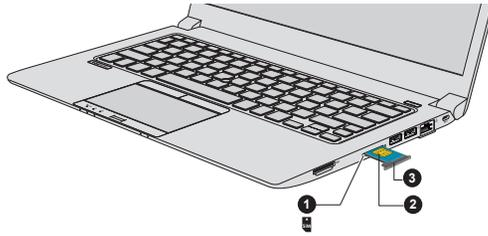
Figure 4-7 Installing the SIM Card (Z40-C)
