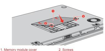
Figure 4-13 Seating the memory module cover
