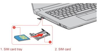
Figure 4-10 Installing the SIM Card (A40-C/R40-C)
