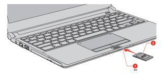
Figure 4-19 Inserting memory media (A40-C/R40-C)
