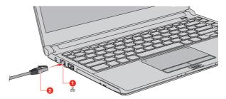
Figure 4-16 Connecting the LAN cable (A40-C/R40-C)
