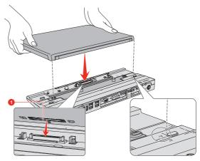
Figure 4-23 Aligning your computer with the Port Replicator (A40-C)
