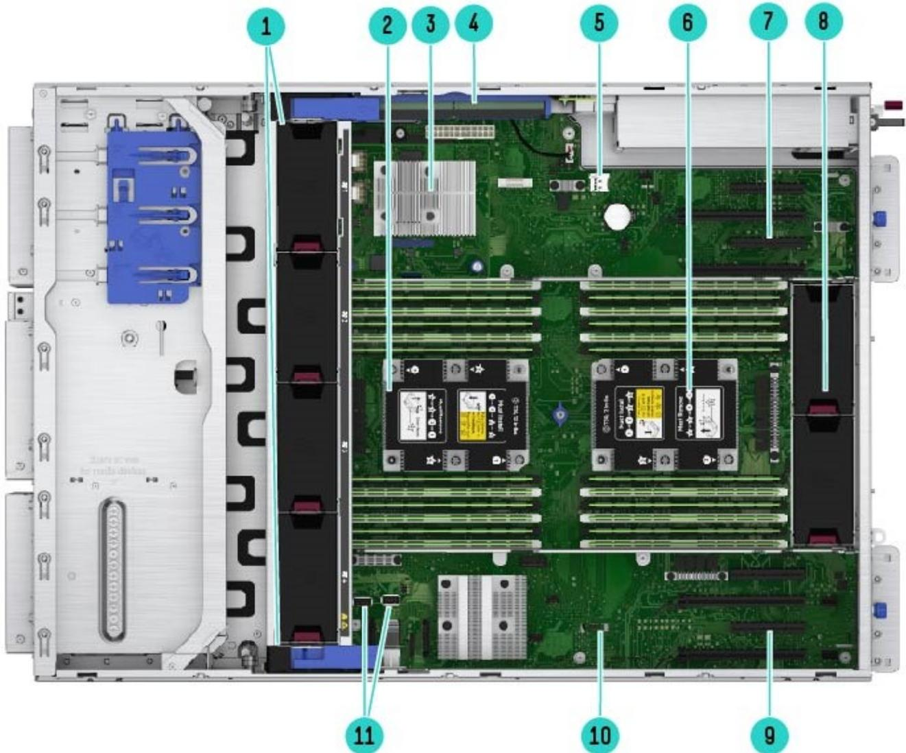
**Internal View – with optional 2<sup>nd</sup> CPU, Smart Array Modular Controller and Redundant Fan Kit shown**
