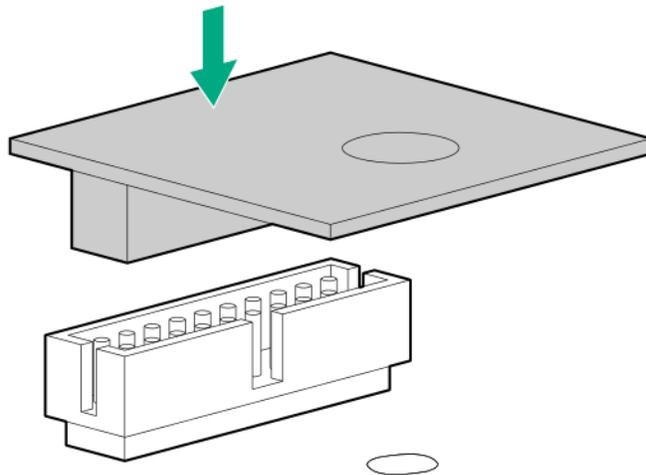
3. Install the TPM security rivet by pressing the rivet firmly into the system board.
