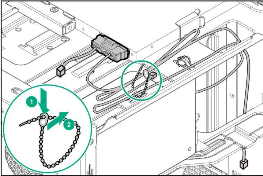
c. Connect the power end of the SATA cable to the power supply cable labeled P3.
