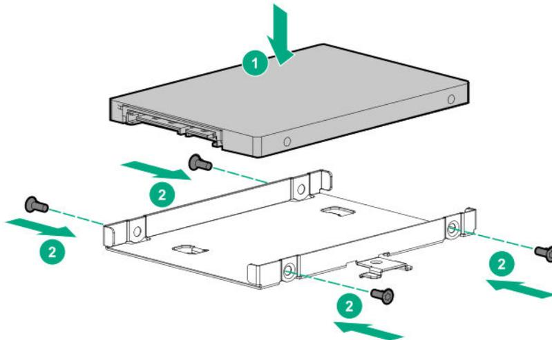
2. Install the SSD assembly in the media bay, and then secure it with the screw.
