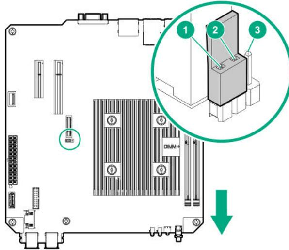
7. After five seconds, remove the jumper from pins 1 and 2, and move it back to the default position on pins 2 and 3.
