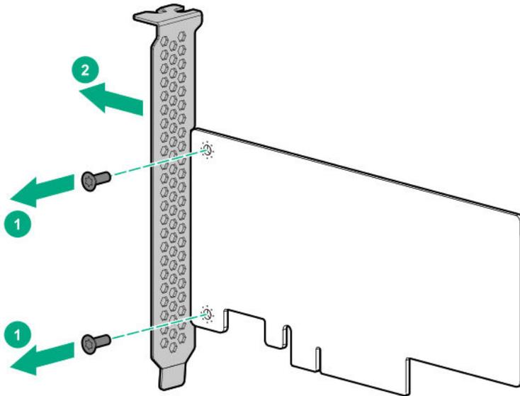
2. Install the low-profile bracket on the expansion board.
