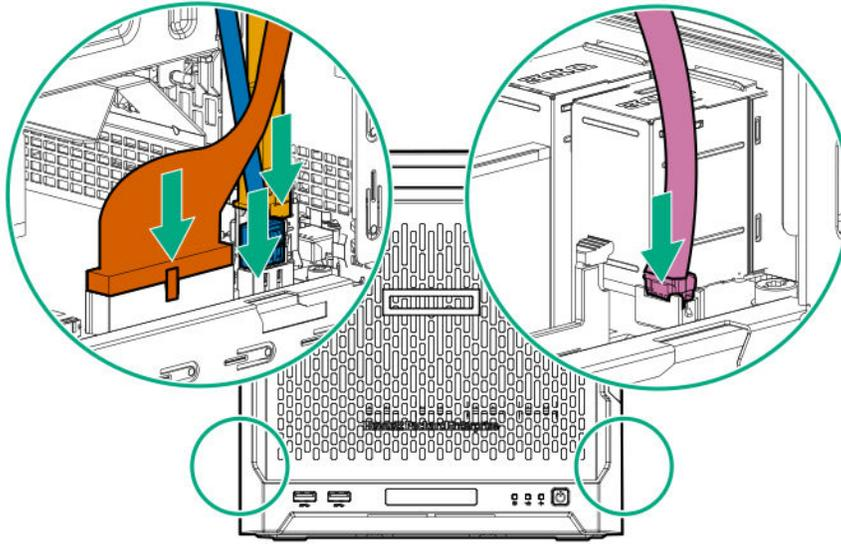
5. If removed, install the internal USB device.
