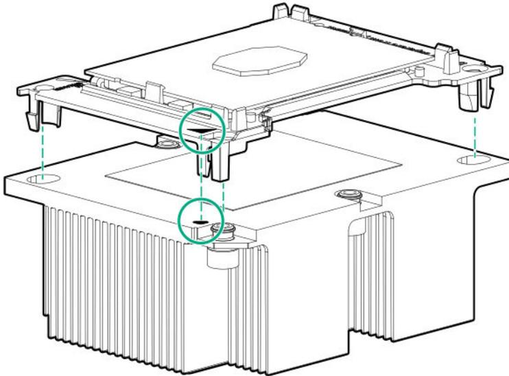
11. **Install the processor heatsink assembly.**
