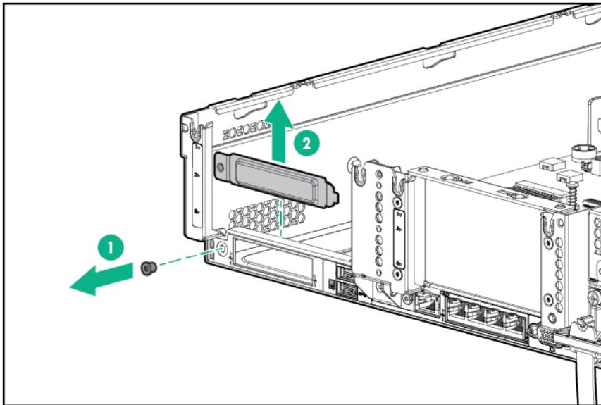
7. Install the FlexibleLOM adapter:
