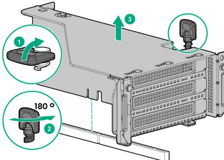
Remove the secondary wall blank.
