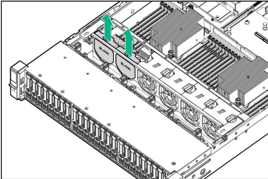
4. **Remove the air baffle.**
