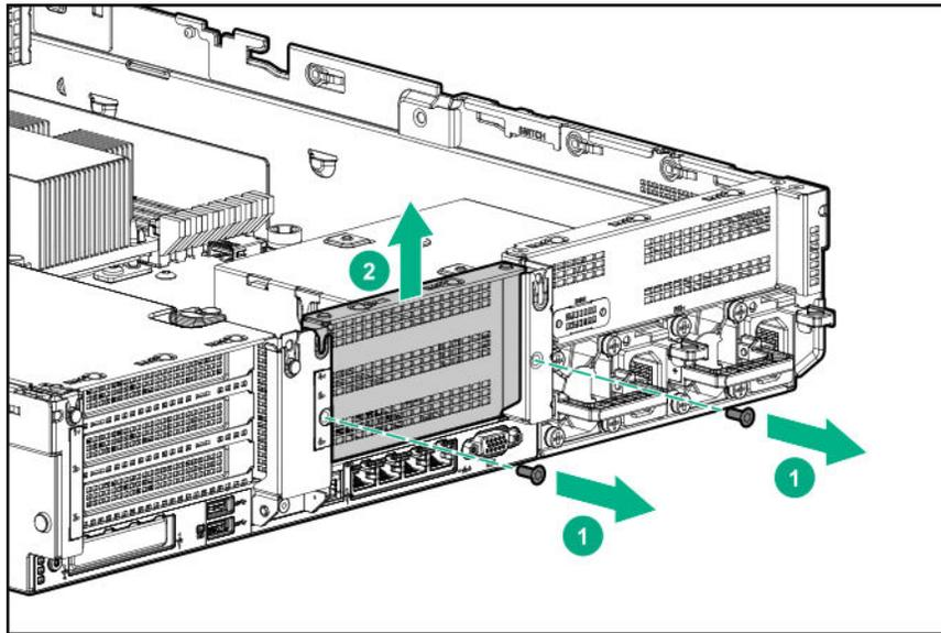
To install a card in the primary riser cage, see "[Removing a riser cage](#)".
