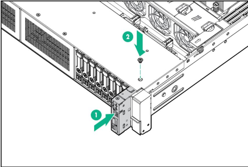
10. Connect the SID module cable to the front power/USB 3.0 connector.
