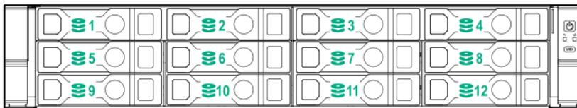
When any stacked 2SFF drive configuration is connected to the SAS expander, the drive numbering skips the second number to allow **uFF drive bay numbering** on page 36.
