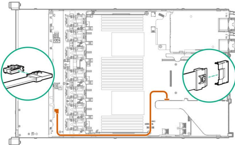
13. Install the primary PCI riser cage.
