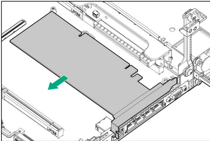
10. Remove the PCI riser cage.
