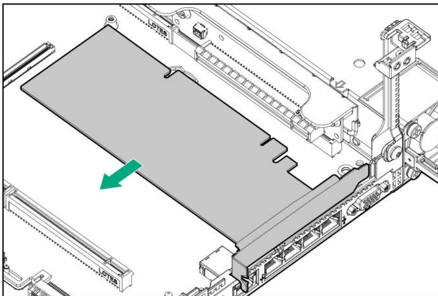
9. Remove the primary PCI riser cage (**Remove the primary PCI riser cage** on page 35).
