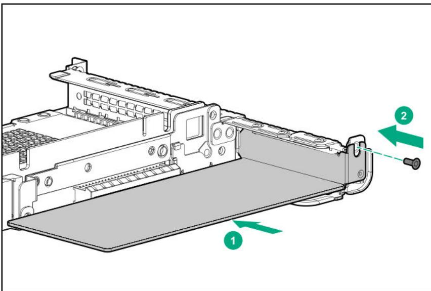
10. Install the primary PCI riser cage (**Install the primary PCI riser cage** on page 36).
