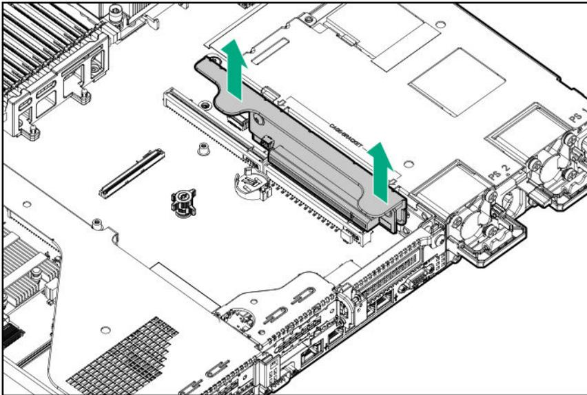
8. Install the secondary full-height PCI riser cage (**Installing a secondary full-height PCI riser cage option** on page 91).
