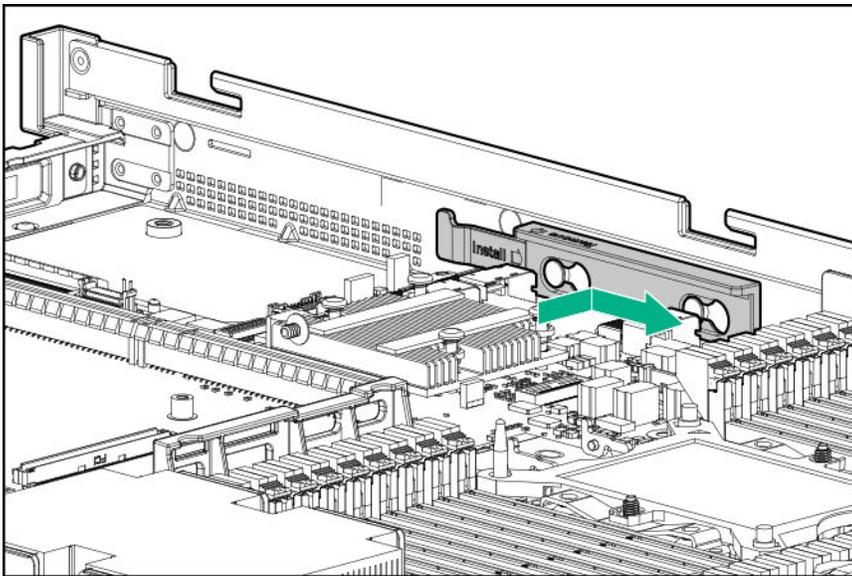
11. Install the riser cage ([Install the primary PCI riser cage](#) on page 36).
