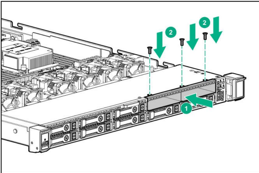
8. Remove the primary PCI riser cage (**Remove the primary PCI riser cage** on page 35).
