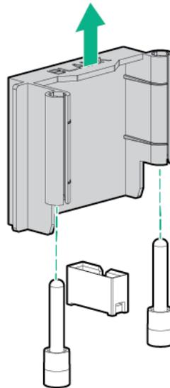
8. Install high-performance fans in each of the seven fan bays.
