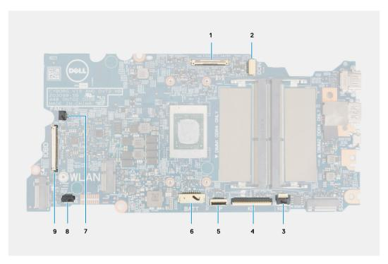
Figure 2. System board connectors
