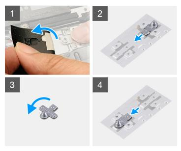
The following image provides a visual representation of the procedure to install the solid-state drive mounting bracket when replacing M.2 2280 solid-state drive with M.2 2230 solid-state drive in M.2 slot one.
