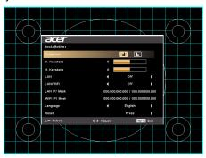
3 The background pattern acts as a guide to adjusting the calibration and alignment settings, such as screen size and distance, focus and more.
