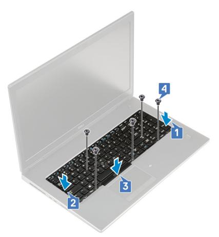
d Align the keyboard lattice to its position on the keyboard and ensure that the keyboard lattice clicks into its place.
