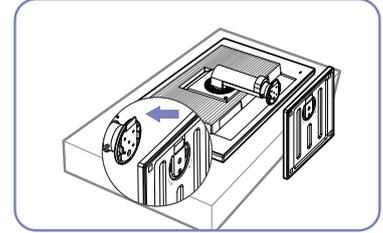
Insert the stand base into the stand in the direction of the arrow.
