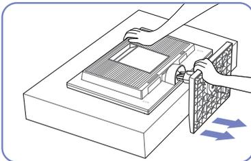
While holding the stand neck with one hand, pound the other fistful hand down onto the top of the stand base in the direction of the arrow to detach the stand base.
