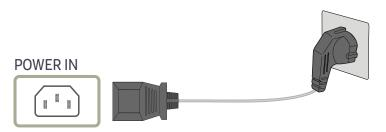
To use the product, connect the power cable to a power outlet and the **POWER IN** port on the product.
