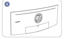
A Attach the BRACKET WALL here
