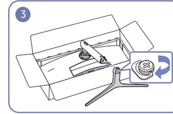
3 Insert the stand base into the stand neck in the direction as shown in the figure.
