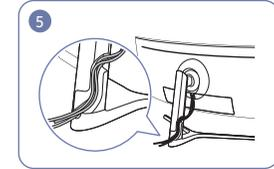
Place the corresponding cables into the stand-neck holder. Do not stretch the cable. Three cables in one holder is recommended.
