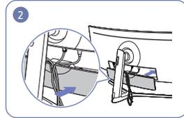
Arrange the cables against the bend tendency of the cables and pull the cables out of the COVER-REAR SUB grooves.
