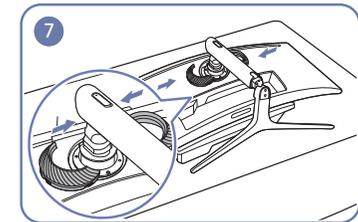
7 Assemble the COVER-REAR TOP to the stand neck as shown in the figure.
