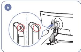
Attach the COVER STAND BODY REAR in the direction as shown in the figure with the buckles not being exposed.
