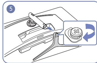
5 Insert the stand base into the stand neck in the direction as shown in the figure.
