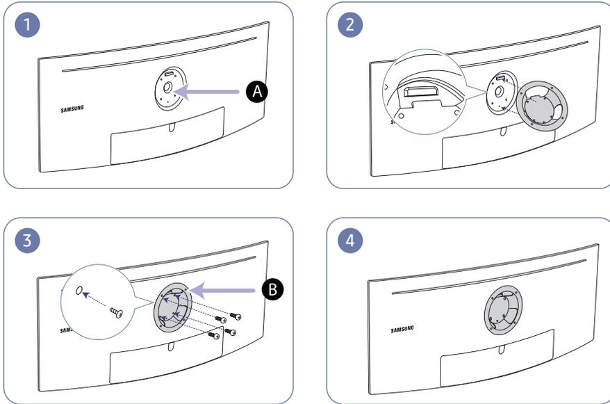
**A** Attach the BRACKET WALL here
