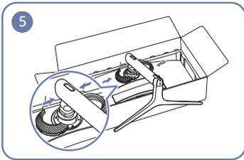
5 Assemble the COVER-REAR TOP to the stand neck as shown in the figure.
