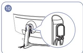
Arrange the cables against their bend tendency, and then pull them through the HOLDER-CABLE hangers. When the set height is changed, you need to arrange the cables and pull them through the HOLDER-CABLE hangers again.
